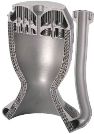
ROCKET PROPULSION ENGINE - SLM® 280 Twin - IN718 built with 400W lasers at 30µm - 개당 2일 18시간 소요
